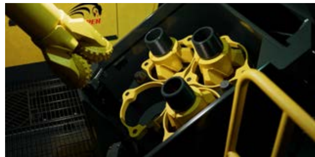
The Automatic Bit Changer (ABC) enables hands-free bit changes and enhances productivity and safety by eliminating human interaction with the drill string. Following the positive customer feedback from the introduction in the Pit Viper 270 series, Epiroc has extended the solution to the popular Pit Viper 351 blasthole drill rig.
